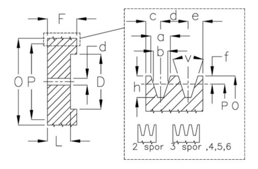
$\begin{array}{lll} D & = 103 \\ d & = 20 \\ F & = 85.0 \\ L & = 65 \\ Number of ribs = 3 \\ O & = 169.6 \\ P & = 160 \\ Type & = C \\ \end{array}$
